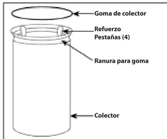
Fig. L – Colector
